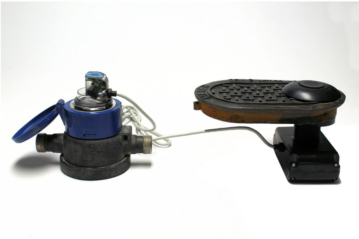
*Figure 5 CYCLOPS Camera End Module and MIU with Thru Lid Implementation*
