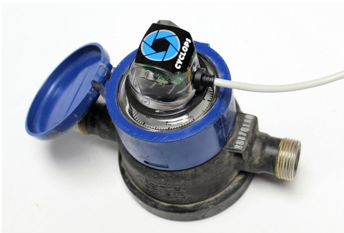
*Figure 3 CYCLOPS Camera End Module, 100% Sealed Register Mounting, with Clear Reading Window*
