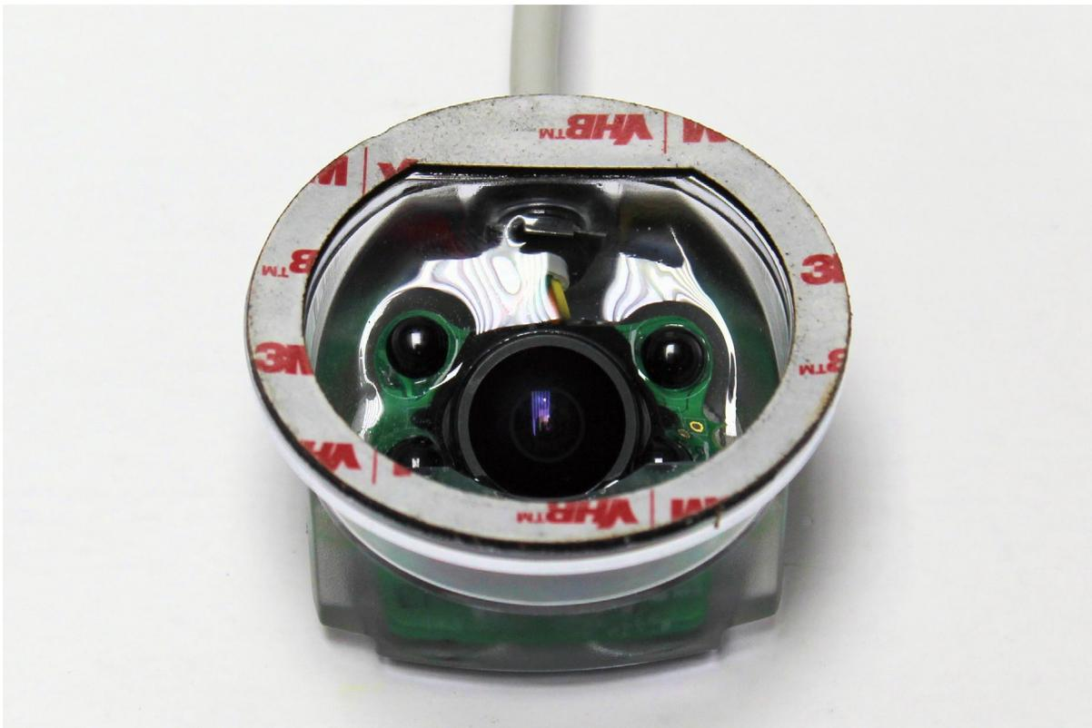
*Figure 4 CYCLOPS Camera End Module (underside), Potted Components, High Bond Adhesive*
